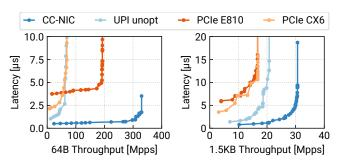
**Figure 11.** Throughput-latency curves, comparing CC-NIC, unoptimized UPI, and PCIe loopback performance on the ICX server, for 64B and 1.5KB packet sizes
