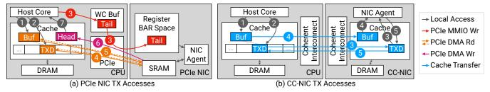
Figure 4. Comparison of TX path accesses for (a) the Intel E810, and (b) the CC-NIC interface. Numbers denote access order.
