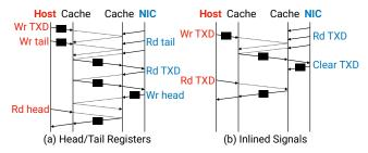
**Figure 6.** Signaling communication with (a) registers, and (b) signals inlined in the descriptor. Dotted lines represent coherence metadata.
