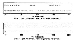
Fig. 4. Comparisons between Tcplib and exponential interpacket times.
