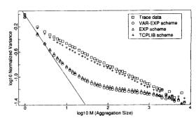
Fig. 5. Variance-Time Plot for TELNET packet arrival process. The line from the upper left corner has slope -1.
