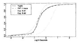
Fig. 3. Empirical distributions of packet-interarrivals within TELNET connections.
